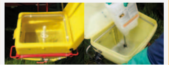
Induction hopper & Container cleaning process
